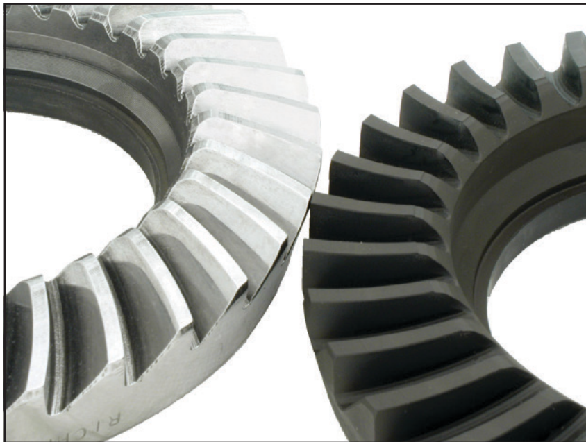
A Comparison of a standard ring gear and a ISF/Supra-Fin processed gear. Photo Courtesy of Mark Williams Enterprises.
