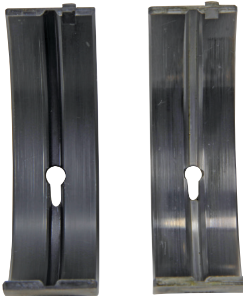
Judge for yourself. Both Federal-Mogul/Speed-Pro main bearings shown above had approximately 100 drag racing passes on them prior to removal and came from the same engine. The bearing on the left was dry film lubricant coated by Calico Coatings, while the bearing on the right was untouched.
